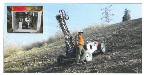
voir (VVR). TEI installed Smart Reservoir's VVR-400 to solve hydraulic issues with its drill prototype. The VVR was chosen due to its compact size, low weight and ability to supply the hydraulic pump at extreme angles. With a standard reservoir, at certain angles the inlet to the pump may become uncovered, leading to starving of the pump; the constant pressure provided by the VVR solves this issue.
